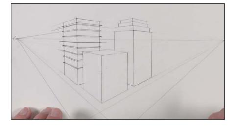
We'll add a few rows of windows on our first building. On the right side of the corner, we'll use the right vanishing point to establish the angled lines. For each window edge, vertical lines are used. Be sure that these lines are vertical and are parallel to the corner.
