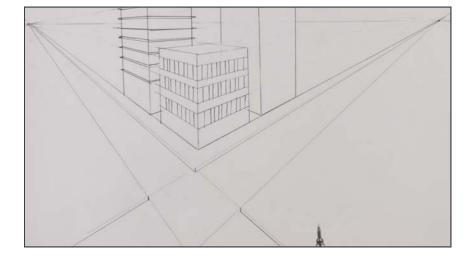
Cracks are added to the sidewalk by drawing lines to the opposite vanishing point. These lines should be drawn closer together as they recede back in space.
