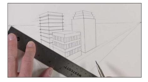
We'll add a couple of additional lines for a sidewalk and add some dimension to it with a curb. A vertical line is used to establish the corner of the sidewalk curb with lines that recede from its bottom to each of the vanishing points.
