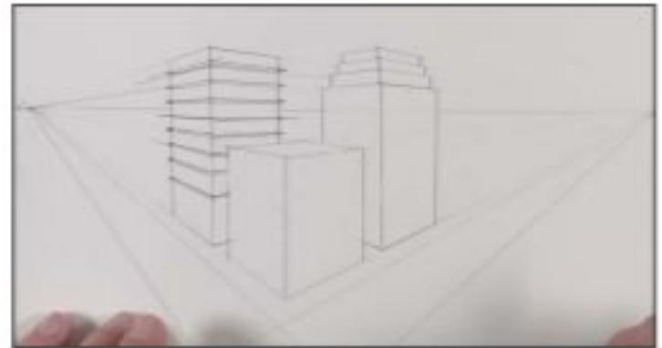
We'll add a few rows of windows on our first building. On the right side of the corner, we'll use the right vanishing point to establish the angled lines. For each window edge, vertical lines are used. Be sure that these lines are vertical and are parallel to the corner
